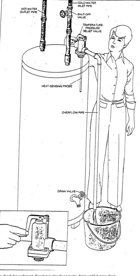
bottom of the tank is the drain valve, to check for sediment. If water is cloudy or rusty, drain until it runs clear.
